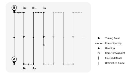
Lengthen or shorten AB Route: Shorten the AB route, Fly from point B to point A, when approaching target point, keep pulling the right joystick downward. After the route is shortened, return the joystick to the center. Lengthen the AB route, you can push the right joystick upward when approaching target point. After the aircraft arrive at the target point, then return the joystick to the center.
