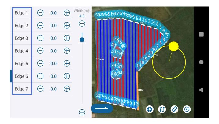
C. Tap one of the plot corner on the map to set the starting point. The Route Width, Route type, Maximum mileage, Safety Dis and Obstacle safe Dis accordingly.
