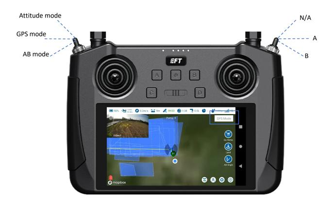
2. In spray mode, tap the C and D buttons (The switch button is user-definable) to turn on the water pump and nozzles respectively to check if they are working properly.
