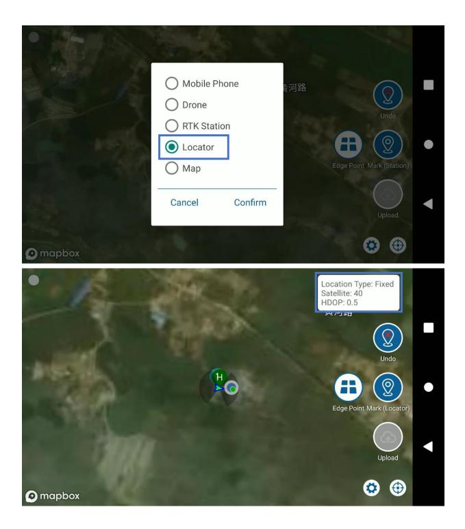
d. Hold the dotting device and walk to the boundary of the plot to set dots. If there are obstacles, tap
