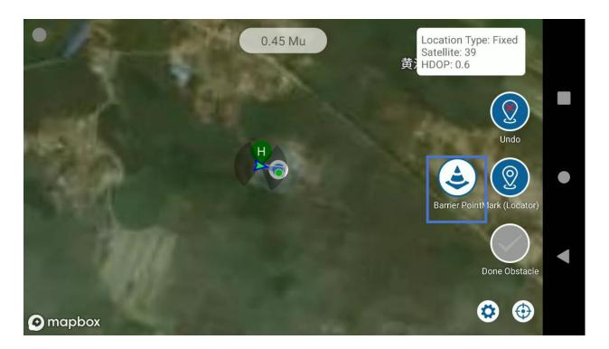
e. Obstacle dots can be set as polygon or circle. and tap the icon to adjust the margins Then Done Obstacle to save it.
