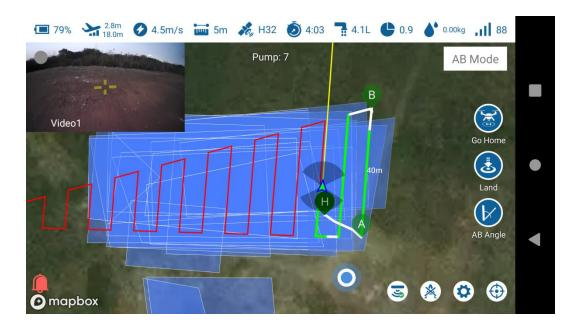
Interrupt/ Continue AB route: Switch the flight mode of the left lever to interrupt the operation at AB mode. If you want to return to the breakpoint, after takeoff in GPS mode, switch to AB mode again, and the drone will automatically return to the breakpoint to continue work.
