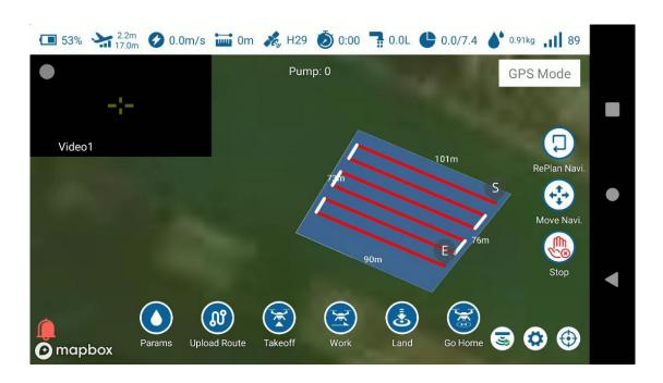
Tap Params to set Hight, Speed and Quantity, tap Upload Route and Make sure Navi-points is ok, Then tap Takeoff and After flying up, tap Work to start spraying automatically.
