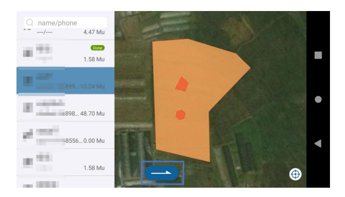
b .Tap the **Edge** to adjust the route direction ,and adjust the safety distance of each route by - or +.
