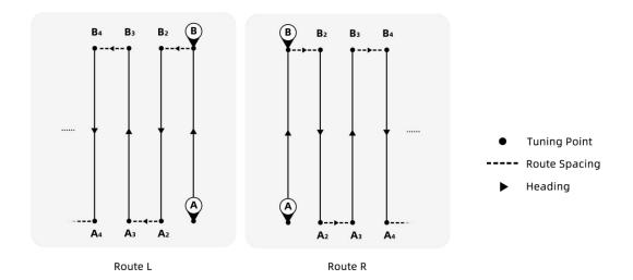
Adjust AB angle: After setting point A, rotate the drone head to align with the target direction. Tap the AB Angle button to record the angle of point A. Record point B in same way after setting point B.
