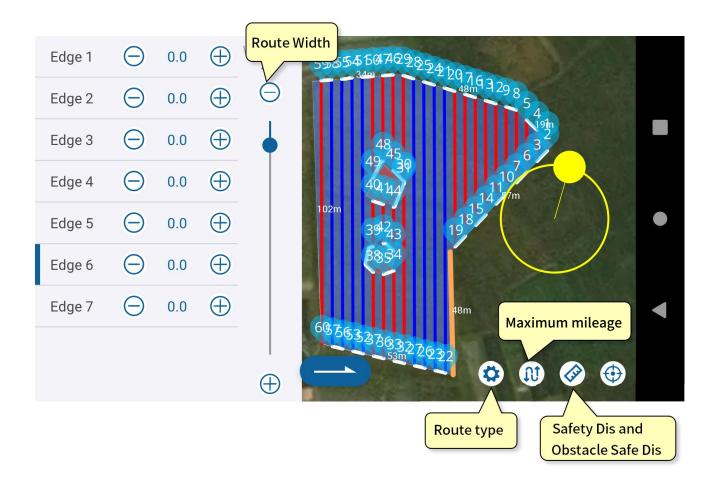
d. Tap , choose the Route type as U-Type /Along side /Tree-Type/Throwing. You can also adjust the route angle through the ring on the map.
