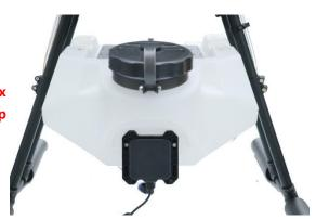
6. Finished front obstacle avoidance radar.
