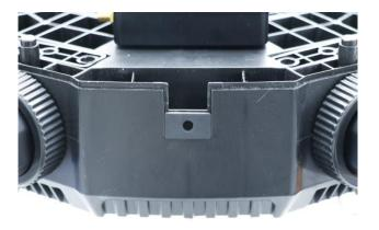
18. The camera harness passes through the wire hole, and the adapter is installed in the card slot.
