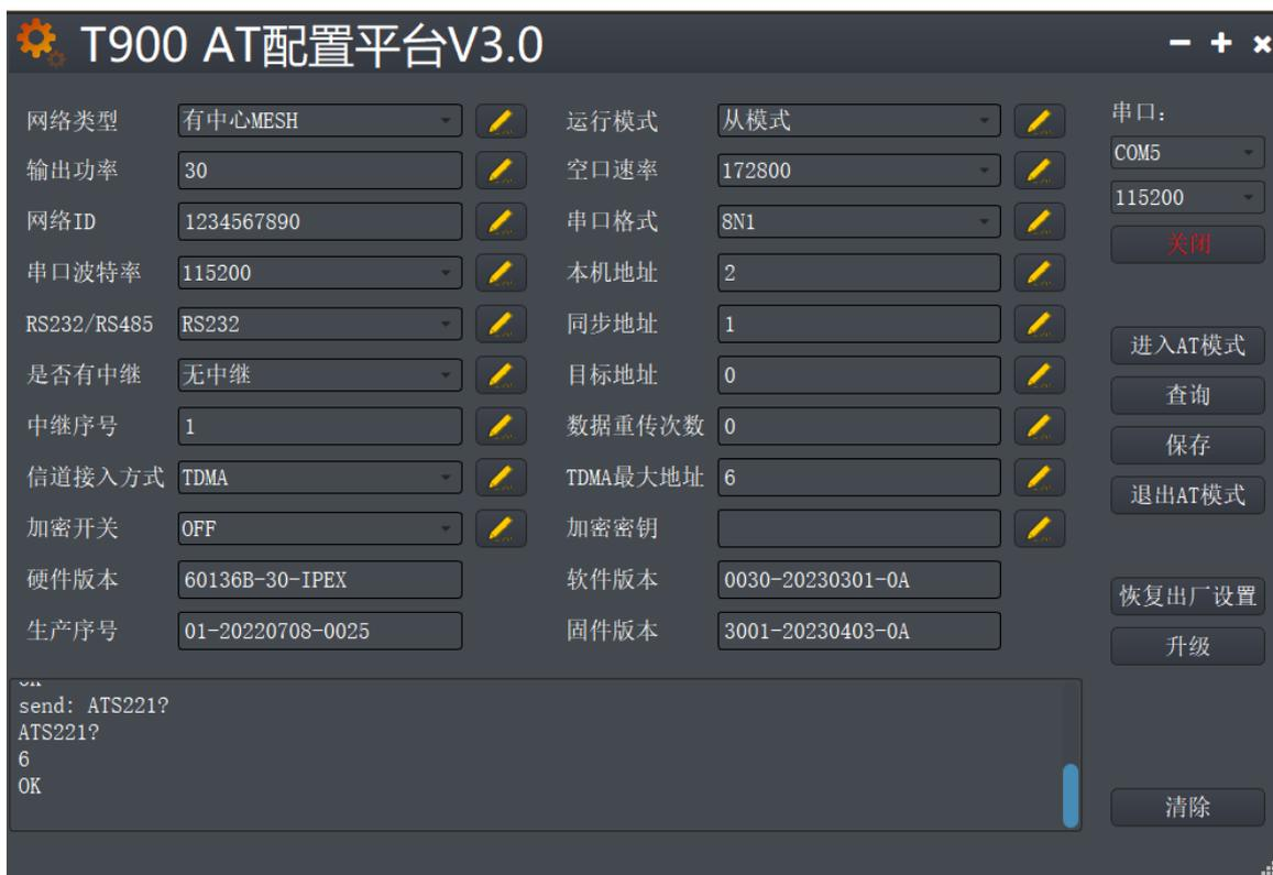
1) Power on the data transmission station, then connect the data serial port, and enter the AT configuration platform.
