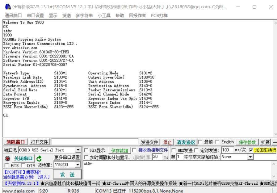
You can use the general serial port terminal, through the data serial port, and use the AT command to configure parameters. For details about how to configure the AT command, see Chapter 6 of the T900 User Manual. Chapter 5 of the T900 User Manual describes how to enter the AT command mode.
