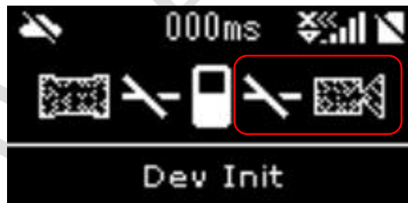
Figure 4- 5 HDMI not connected to the device status
