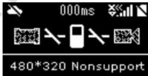
Figure 4-7 HDMI not connected to the device status
