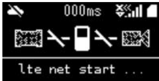
Figure 5-5 4G network connection request
