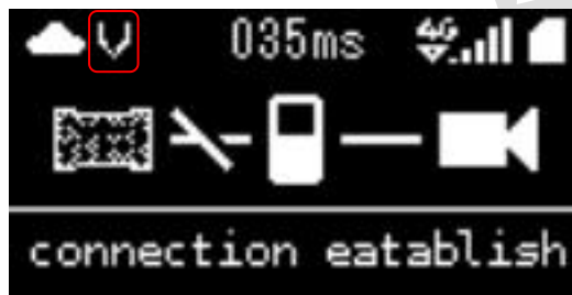
Figure 5-14 Transmitting video data status
