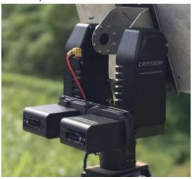
2. The antenna has to be mounted on the Crossbow AAT with the use of a special bracket. In order to prevent tampering with the normal operation of the compass built into the Crossbow AAT it is recommended to avoid using antennas made with ferromagnetic materials. Wherever possible, use non-magnetic stainless steel bolts, aluminum and other non-magnetic materials.
