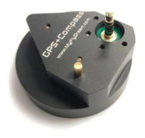
The Crossbow will recognize the GPS+Compass module once it's plugged. The screen will display something like GPS:12/L14 to show the number of satellites locked by remote GPS/ local GPS. With this module, The tracker will start to track when it locks enough satellites without setting home operation.
