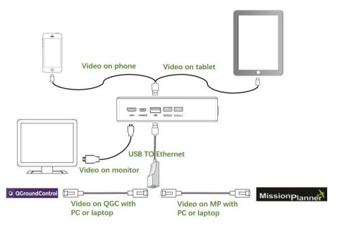
The ground unit outputs video to the monitor via HDMI cable, or you can connect the ground unit to the mobile phone or tablet via USB cable, and opens Viulinx APP to watch the video. QGC is also supported.
