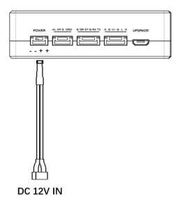
**Pin-out:** - - + +. Insert the four-pin connector of supplied power cable to the power port of the air unit and connect the orange power connect of supplied power cable to a battery output, or the power supply port of a drone. Recommended voltage is 12V.
