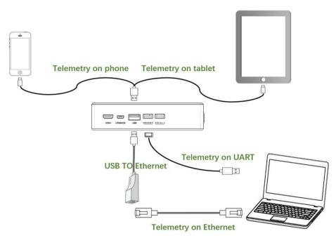
Insert the six-pin connector of supplied serial cable to the serial port of the ground unit and connect the other end of supplied serial cable to the telemetry port of the ground control station.
