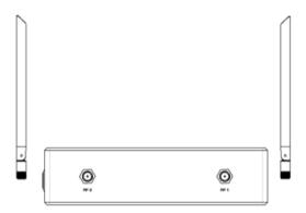
Screw the ground unit antennas onto the RF ports. Make sure the antennas are tightly installed.
