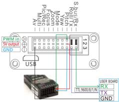
S.bus/Rx: connect to Rx2 for track function.
